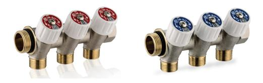
The introduction of the self-sealing O-Ring to the head connections of the manifold and the special synchronization of male/female threads allow the installer to assemble the modules with extreme ease and without the aid of special tools. The alignment of the modules and the hydraulic hold are in this way easily guaranteed and reliable.
