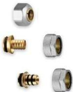
**208 – 216T – 217T** Compression fittings with nut threaded 3/4" Eurocone, to connect copper pipes, polyethylene pipes and multilayer pipes at the manifolds. Available for the main commercial sizes of pipes
