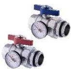
**305NTK/1** Pair of straight full port ball valves, with union connection with O-Ring seal, completed with thermometer scale 0÷80°C. Available sizes 1" and 1-1/4".
