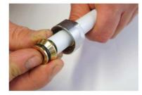
Insert completely the body of the fitting into the pipe exerting an enough pressure, and paying attention to don't damage or move the two O-ring
