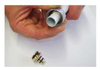
Insert the nut with pre-assembled retaining ring on the pipe to connect
