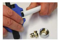
After cutting the pipe in a clear manner perpendicular to its axis, calibrate and deburr it with an appropriate tool
