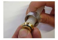
Insert completely the body of the fitting into the pipe exerting an enough pressure
