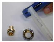
Cut the pipe with a shear cleanly and perpendicularly to its axis
