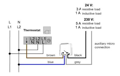
The power supply connection is the same for all models. The scheme show the types with micro switch four wires
